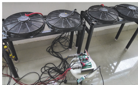
FIGURE 9: In lab bench test of the ECU control system.
